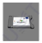
CAM is Conditional Access Module with common conditional access interface (Common Interface) in TVs and digital television receivers. The CAM allows to provide subscribers with access to encrypted content in digital television.
