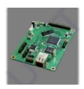
DVB IP input/output board is designed for receiving/transmitting the DVB TS using UDP / RTP protocols accordingly to DVB-over-IP standard including converting from/into synchronous parallel interface.
