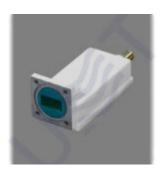
Ku-band LNB DRO LO 13.05 is Low Noise Block Down Converter with single LO 13.05 GHz and single 75 Ohm F-type output. LO instability: ± 2 MHz, Gain: 58 dB, Noise figure: 0.9 dB, Output power P1dB: +3 dBm.
