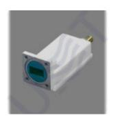
Ku-band LNB DRO LO 9.75 is Low Noise Block Down Converter with single LO 9.75 GHz and single 75 Ohm F-type output. LO instability: ± 2 MHz, Gain: 58 dB, Noise figure: 0.9 dB, Output power P1dB: +3 dBm.
