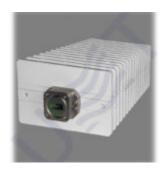
BUC-Ku20-11.3 v2 is block up-converter with fixed output power P1dB **20 W** (ALC power: 2000 mW) and LO of **11.3 GHz**.
