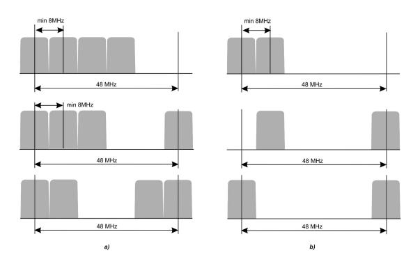
Examples of packages spectrum arrangement within 48 MHz of 4RF (a) and 2RF (b)
