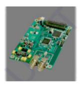
2 ch DVB-S-S2 receiver board is designed to convert the DVB-S/S2 IF (intermediate frequency in the L-band obtained from the LNB) to parallel DVB TS (transport stream).
