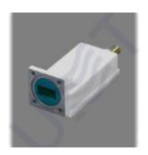
Ku-band LNB DRO LO 10.60 is Low Noise Block Down Converter with single LO 10.60 GHz and single 75 Ohm F-type output. LO instability: ± 2 MHz, Gain: 58 dB, Noise figure: 0.9 dB, Output power P1dB: +3 dBm.
