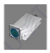
Ku-band LNB PLL LO 10.75 is Low Noise Block Down Converter with single LO 10.75 GHz and single 75 Ohm F-type output. LO instability: ± 150 kHz, Gain: 45 dB, Noise figure: 0.9 dB, Output power P1dB: +3 dBm.
