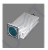
Ku-band LNB PLL LO 11.80 is Low Noise Block Down Converter with single LO 11.80 GHz and single 75 Ohm F-type output. LO instability: ± 150 kHz, Gain: 45 dB, Noise figure: 0.9 dB, Output power P1dB: +3 dBm.
