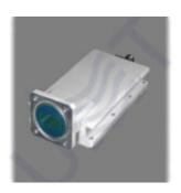
Ku-band LNB PLL LO 8.80 is Low Noise Block Down Converter with single LO 8.80 GHz and single 75 Ohm F-type output. LO instability: ± 150 kHz, Gain: 45 dB, Noise figure: 0.9 dB, Output power P1dB: +3 dBm.
