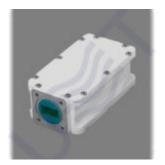
Ku-band LNB PLL with AGC LO 12.80 is low noise block down converter with automatic gain control. It is professional LNB with wide dynamic range – up to 50 dB (biggest among any other LNB). AGC range: 20 dB, LO instability: ±25 kHz, Gain (min): 34 dB.
