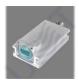
PLL LNB with AGC L.O. 10.45 is professional low noise block down converter with automatic gain control, wide dynamic range of up to 50 dB (biggest among any other LNB). AGC range of 25 dB, LO instability of 50 kHz, Gain (min) of 40 dB.
