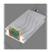
PLL LNB with AGC L.O. 12.8 is professional low noise block down converter with automatic gain control, wide dynamic range of up to 50 dB (biggest among any other LNB). AGC range of 25 dB, LO instability of 50 kHz, Gain (min) of 40 dB.
