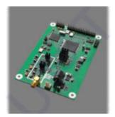
L-band DVB-S-S2-T modulator board is designed for DVB TS (transport stream) modulating, creating the L-band IF signal from parallel TS for further broadcasting in DVB-S, DVB-S2 or DVB-T standards.
