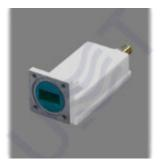
Ku-band LNB DRO LO 10.60 is Low Noise Block Down Converter with single LO 10.60 GHz and single 75 Ohm F-type output. LO instability: ± 2 MHz, Gain: 58 dB, Noise figure: 0.9 dB, Output power P1dB: +3 dBm.
