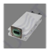
Ku-band LNB PLL dual LO 9.75 10.6 v.2 is Low Noise Block Down Converter with dual local oscillator 9.75 GHz and 10.6 GHz and dual 50 Ohm N-type output. LO instability: ± 2.5 ppm, Gain: 55 dB, Noise figure: 0.8 dB, Output power P1dB: 0 dBm.
