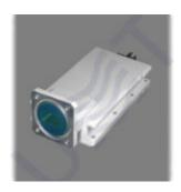
Ku-band LNB PLL LO 10.60 is Low Noise Block Down Converter with single LO 10.60 GHz and single 75 Ohm F-type output. LO instability: ± 150 kHz, Gain: 45 dB, Noise figure: 0.9 dB, Output power P1dB: +3 dBm.
