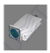
Ku-band LNB PLL LO 12.80 is Low Noise Block Down Converter with single LO 12.80 GHz and single 75 Ohm F-type output. LO instability: ± 150 kHz, Gain: 45 dB, Noise figure: 0.9 dB, Output power P1dB: +3 dBm.
