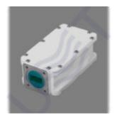
Ku-band LNB PLL with AGC LO 10.6 is low noise block down converter with automatic gain control. It is professional LNB with wide dynamic range – up to 50 dB (biggest among any other LNB). AGC range: 20 dB, LO instability: ± 25 kHz, Gain (min): 34 dB.
