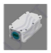
Ku-band LNB PLL with AGC LO 8.80 is low noise block down converter with automatic gain control. It is professional LNB with wide dynamic range – up to 50 dB (biggest among any other LNB). AGC range: 20 dB, LO instability: ± 25 kHz, Gain (min): 34 dB.
