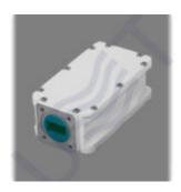
Ku-band LNB PLL with AGC LO 9.75 is low noise block down converter with automatic gain control. It is professional LNB with wide dynamic range – up to 50 dB (biggest among any other LNB). AGC range: 20 dB, LO instability: ± 25 kHz, Gain (min): 34 dB.
