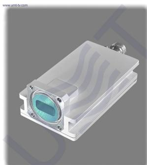
New PLL LNB with AGC L.O. 10.55 is professional low noise block down converter with automatic gain control, wide dynamic range of up to 50 dB (biggest among any other LNB). AGC range of 25 dB, LO instability of 50 kHz, Gain (min) of 40 dB.
