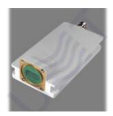
PLL LNB with AGC L.O. 11.8 is professional low noise block down converter with automatic gain control, wide dynamic range of up to 50 dB (biggest among any other LNB). AGC range of 25 dB, LO instability of 50 kHz, Gain (min) of 40 dB.
