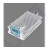
PLL LNB with AGC L.O. 9.75 is professional low noise block down converter with automatic gain control, wide dynamic range of up to 50 dB (biggest among any other LNB). AGC range of 25 dB, LO instability of 50 kHz, Gain (min) of 40 dB.
